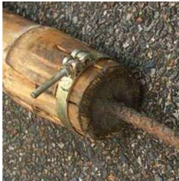
Fig.17 - unión conica - C.Tönges
